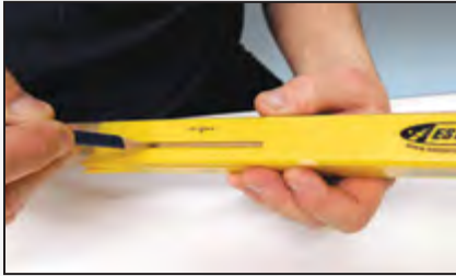
The Tube Marking Guide Allows for Accurate and Consistent Fin Placement When Building Your Rocket.
